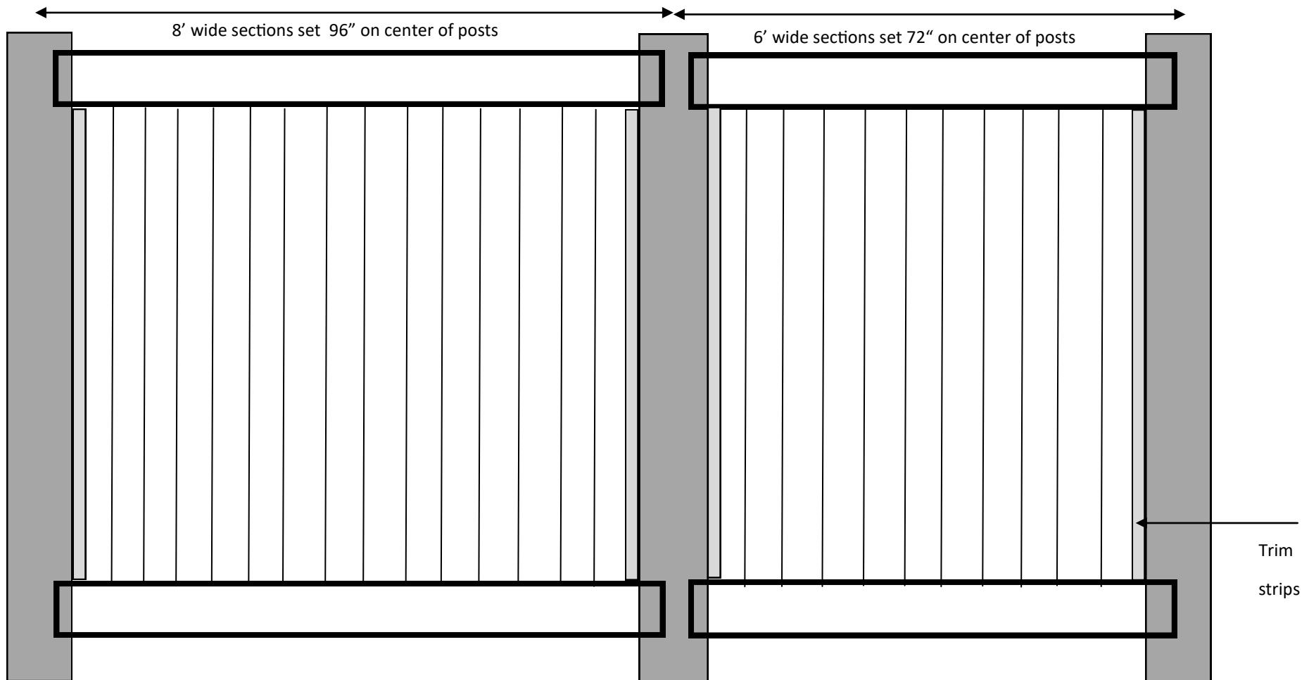
Set posts 24" in ground in cement. FENCE height is to top of post (not to top of rail)
